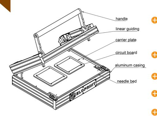
Adaptability through sensors, switches, display elements (LEDs/displays) or switching contact pins for detecting the presence of the test object.
